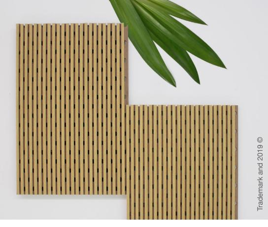
Timberix™ Wooden Grooved panels reduce echoes by trapping and diffracting sound in the grooves and perforation found on the surface. The sound that passes through the perforation is further absorbed by an acoustic substrate such as fibreglass or mineral wool, which reduces reverberation in the room. Smaller grooves are better at attenuating high frequency sounds, whereas larger grooves are better at controlling low frequency sounds.
