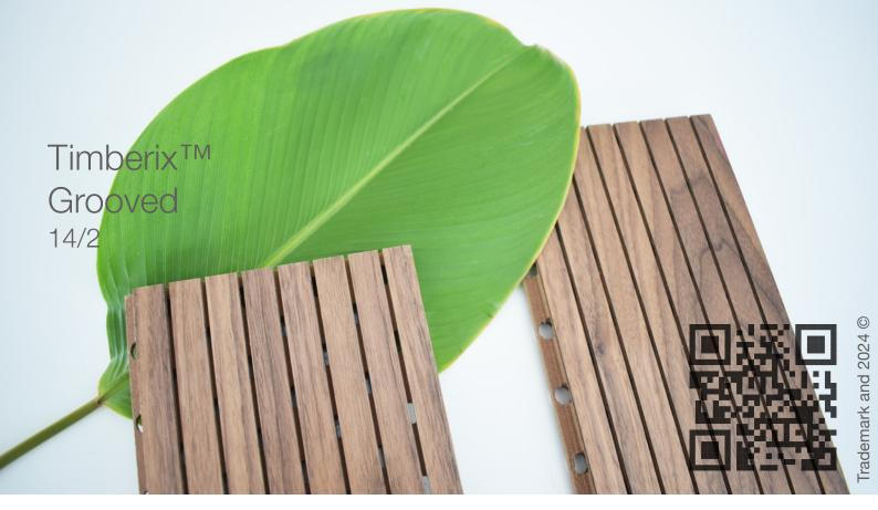
Timberix™ Wooden Grooved panels reduce echoes by trapping and diffracting sound in the grooves and perforation found on the surface. The sound that passes through the perforation is further absorbed by an acoustic substrate such as fibreglass or mineral wool, which reduces reverberation in the room. Smaller grooves are better at attenuating high frequency sounds, whereas larger grooves are better at controlling low frequency sounds.
